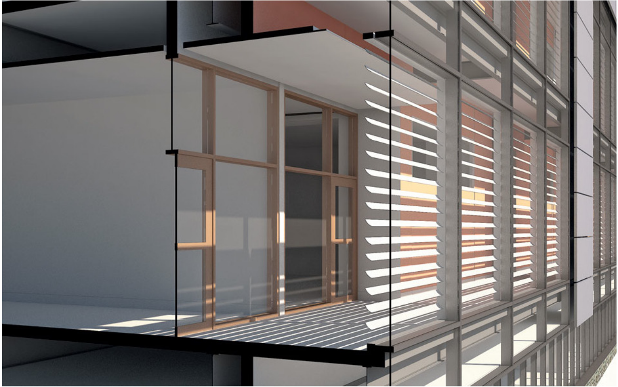
Detail, thermal buffer zone with automated blinds, developed for Brahan Science Center, Hudson Valley Community College, Troy, New York. By Payette.
